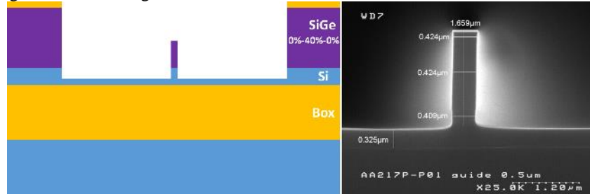
Fig. 1. A schematic of the device structure (left) and scanning electron microscopy (SEM) image of the waveguide.
